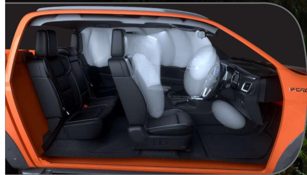
THE NEW D-MAX IS FITTED WITH UP TO EIGHT AIRBAGS
